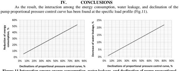
Figure 11 Interaction among energy consumption, water leakage, and declination of pump proportional pressure control curve
