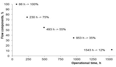
Figure 5 Load profile of network pumps in public water supply system
